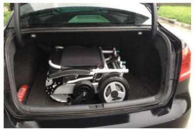
The wheelchair can be folded and placed in the trunk of the car, as shown in Figure. 29. Note: The temperature in the trunk of the car may exceed 50 °C in high temperature weather in summer. At this time, the wheelchair should be taken out in time, otherwise there is a risk of bursting and burning.
