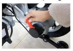
Note: The handle must be pulled up in the electric mode, otherwise the controller will give an alarm and cannot start. In manual mode, the power supply should be turned off, otherwise the push resistance will be very large.
