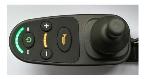
After the user is seated firmly, turn on the power switch and push the joystick knob forward to speed up slowly. If you want to stop, put down joystick knob in your hand and stop. The direction in which joystick knob pushes is the direction in which the wheelchair travels.
