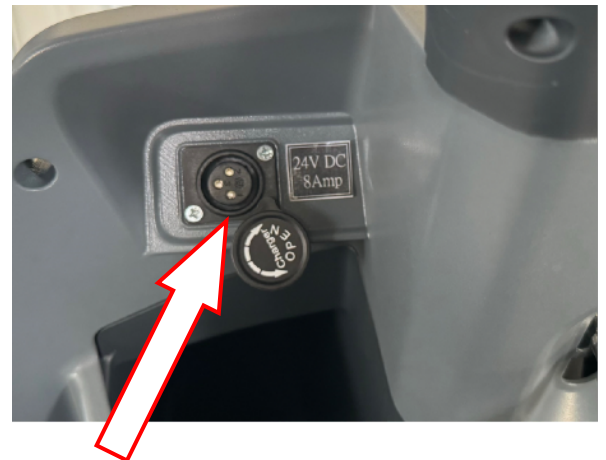
Off-Board Charger Port. The off-board charger port is mounted on the tiller
