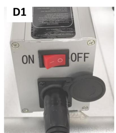
3. In order to prevent the power plug from falling off during use, please fasten the buckle and ensure that the power plug is tightly inserted. Turn on the power switch
