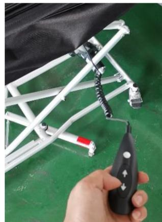
B11. Move the platform car from the vehicle, and ensure that the platform car will not collide with the vehicle during the lowering operation. Keep pressing the Down button on the controller, so that the platform is totally closed.
