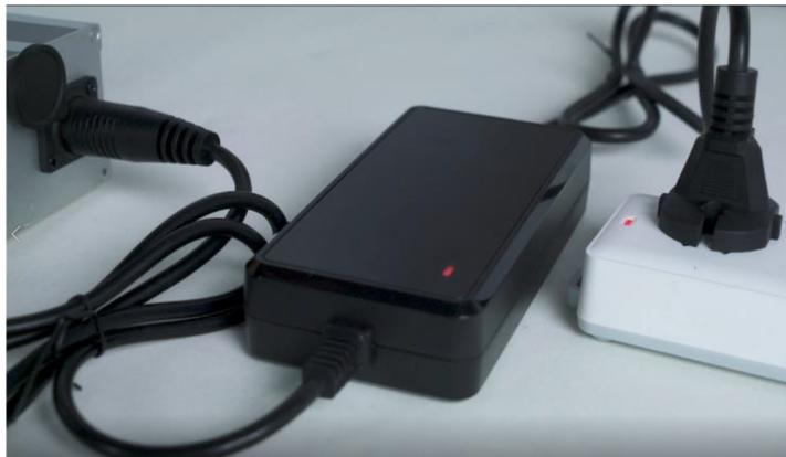
As shown in Figure B, connect one end of the charger to the battery and the other end to the charging plug. The red light on the charger indicates that it is charging and the green light indicates that it is fully charged.
