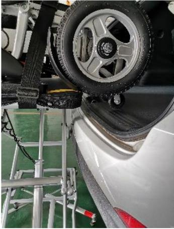
A8. Move the platform to the side of the trunk, adjust the platform height, as shown in the picture, to the height that the anti-overturn small wheel of the wheelchair can go into the trunk...
