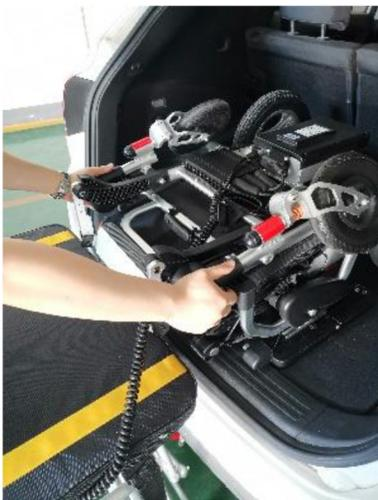
A12. Manually grasp the position in the picture to lift the wheelchair.
