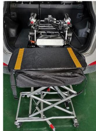
B5. Adjust the position of the platform car, so that the tabletop is 50mm higher than the trunk height. Align the two yellow lines on the platform with the tyres.
