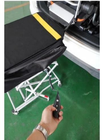
A14. Keep pressing the Down button on the controller, so that the platform is totally closed.
