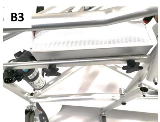
2. Insert the two screws on the battery into the corresponding holes on the frame and tighten the knob. Make sure that the battery is installed in the same direction as Figure B.
