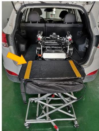
A13. Push it into the trunk, and guarantee that the wheelchair is stably placed. Release the brakes on all castors
