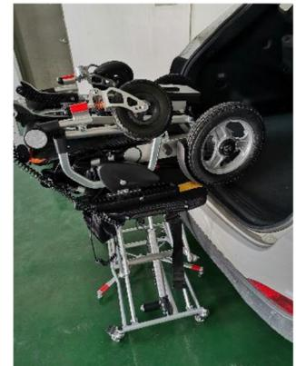
B8. The tyres are in contact with the edge of the tabletop as shown in the picture, to ensure that the wheelchair is stably placed.
