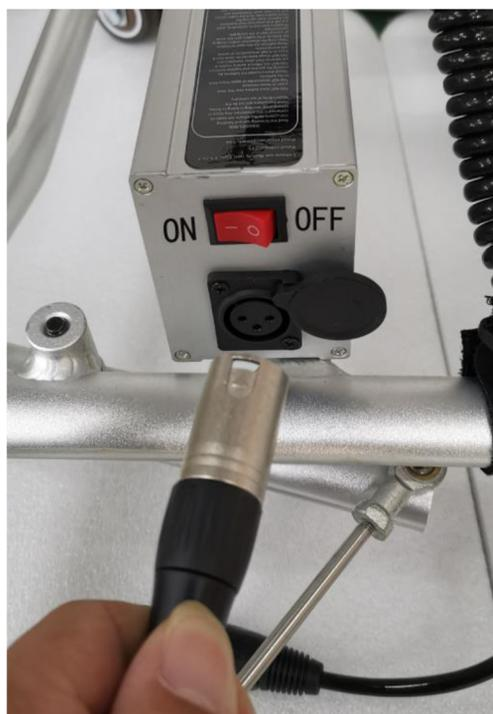
2, If the battery is mounted on the boarding device, you only need to pull out the power plug and insert the charger plug to charge the battery.
